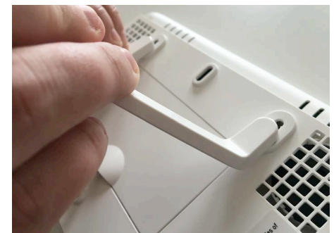
Insert the table stand into the mounting holes and push upward until it snaps into place
